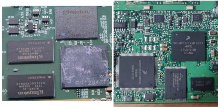
Left: eMMC Flash (BGA) - Right: NAND Flash (TSOP 48)
